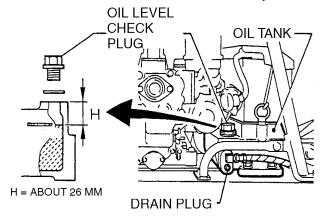
Figure 28. Hydraulic Oil Maintenance
